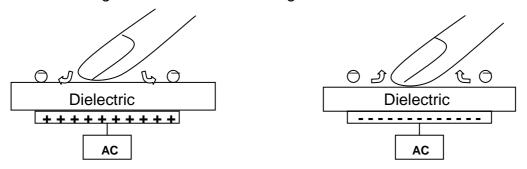
The nature of the ionisation and photon emission is dependent upon a) the nature of the EMF which in this case is constant (10kV impulses of 10 microseconds duration at a repetition frequency of 1024Hz for 0.5 seconds) b) the ability of the object to hold an electric charge (its capacitance) and hence its breakdown voltage c) the nature of the surrounding gases.
